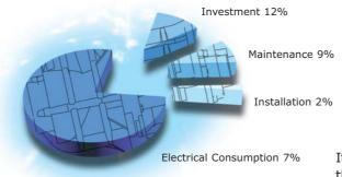
It is well-known that in 3-5 years of operation, over three quarters of the overall cost of a compressor is ascribable to electricity consumption.
