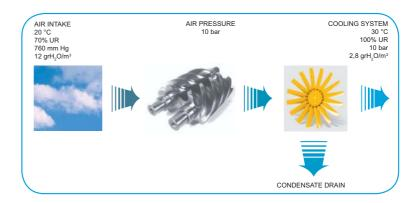
Compressed air is cooled at 30°C and condensed water vapour is separated, while 2.8 gr of water for every Nm³ of air that condense can remain in the air (compressed at 10 bar as in the example) in vapour form.
