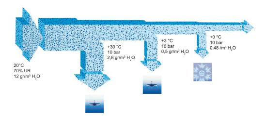
The cooling process does not allow the temperature to fall below  $0^{\circ}$ C (solidification of water). However, specific applications or particular ambient conditions require dew point temperatures of below  $0^{\circ}$ C.
